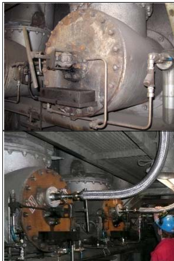
Figure 3. Walking beam furnace at SSAB, Borlänge, Sweden. The original furnace equipped with recuperative air-fuel system (top) and REBOX HLL arrangement (bottom).
