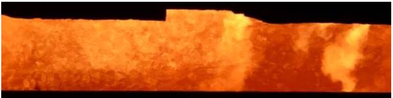
Figure 5. Highly diluted flames created by the REBOX HLL installation at the walking beam furnace in SSAB, Borlänge in Sweden. The fuel used is heavy oil.
