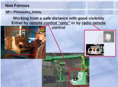
Figure 4: Safety for operator.
