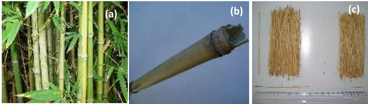
Figure 1. Bamboo trees (a), dried bamboo culm (b) and its fibers longitudinally stripped with different diameters (c).
