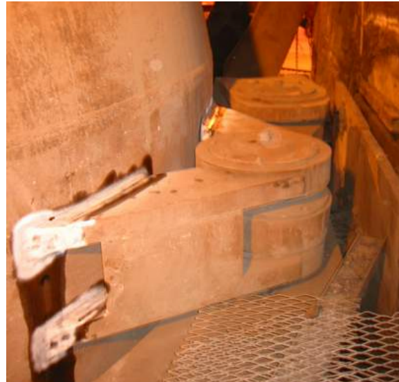
Figure 10: Horizontal link arrangement.
