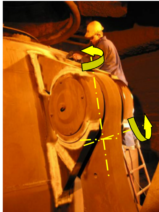
Figure 7: MT of vertical link arrangement. The arrows show possible rigid-body rotations of the link.
