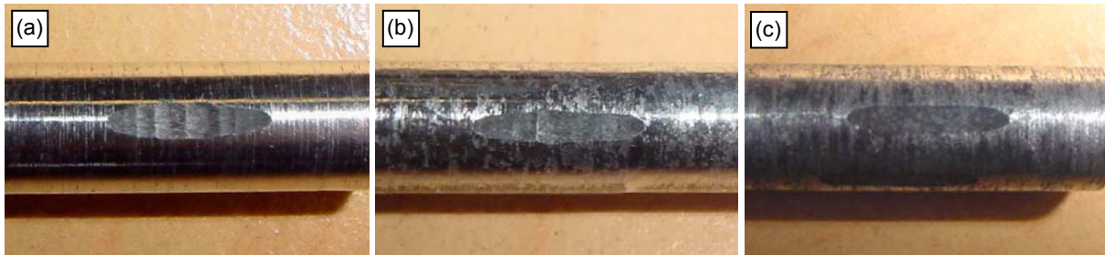
Figure 5. Wear track appearance: (a) A356 matrix alloy, (b) composite 10-35 and (c) composite 10-39-1.
