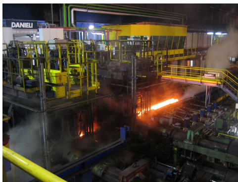
Figure 5 – UFR mill in operation at Arcelor Mittal Differdange (Luxemburg).
