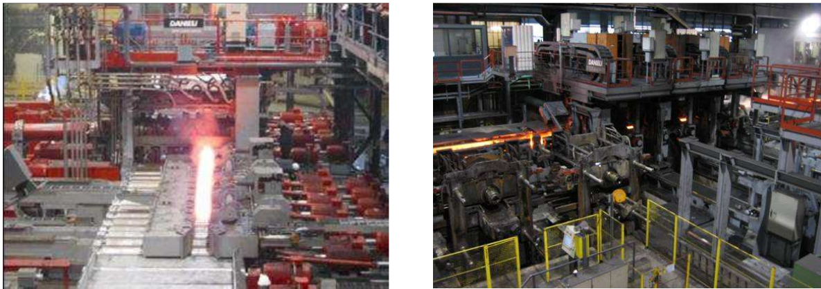
Figure 1 – Break Down mill and UFR finishing mill in operation.
