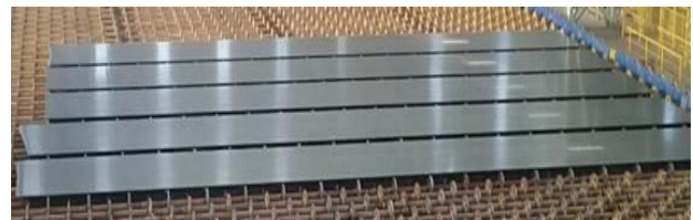
Figure 4: Plates of 25.40 mm in the cooling bed.
