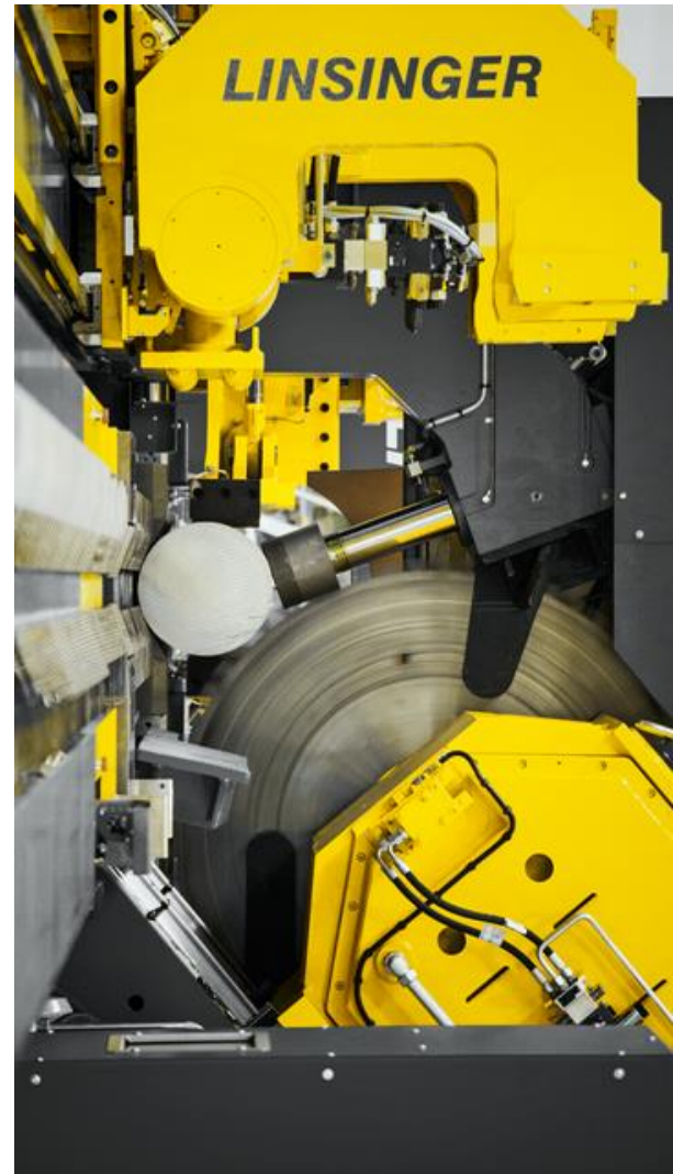
Figure 2. Cutting equipment showing the optimum cutting geometry (applied angle) at KSS 02
