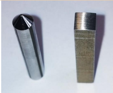
Figure 1. Pins used in the scratch tests (L) and reciprocating sliding tests (R).
