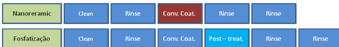
Figure 1 - Comparison of the nanoceramic coating process vs. phosphate coating. (5)
