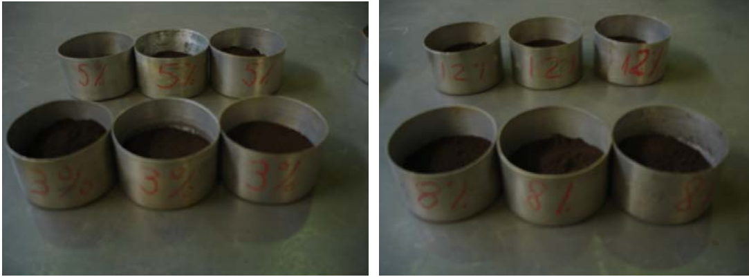
Figure 6 - Detail of the small pots containing the ready materials to be submitted to the compression test (weight % is how much of bonding agent was added into the powder)
