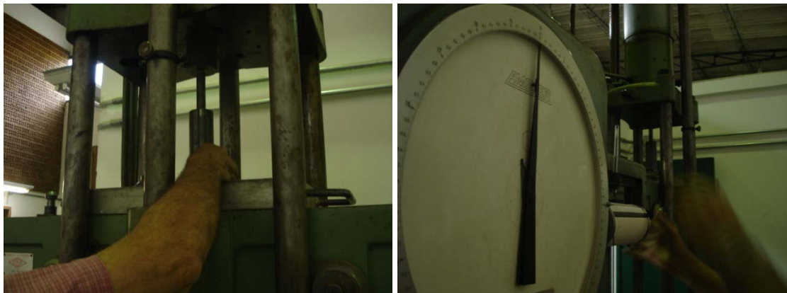
Figure 7 - Detail of the ready matrix to be pressured and the control and register of the adopted load system
