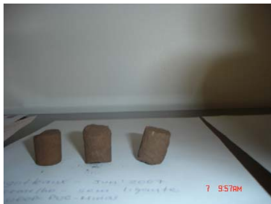
Figure 9 - Photo of the produced briquettes using PUC-Minas' presses
