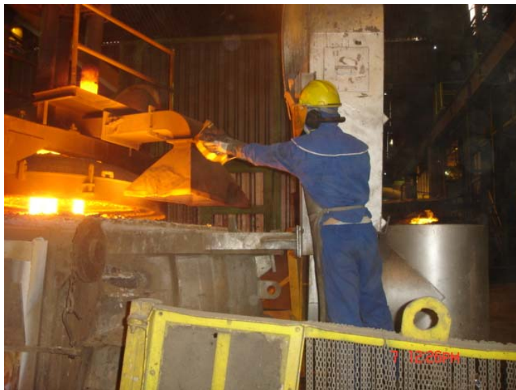
Figure 10 – Addition way in EAF.
