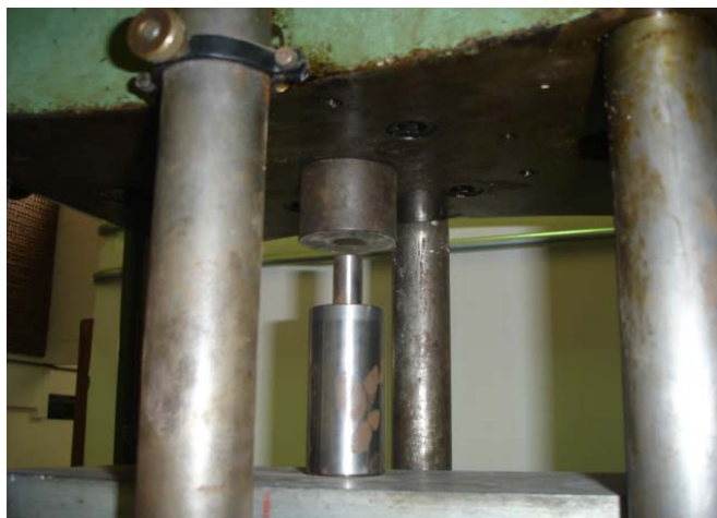
Figure 3 - Detail of the system to pressurize the matrix to produce the briquette.
