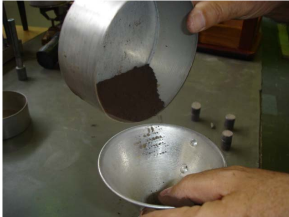
Figure 4 - Dust handling, with mixing and weighting (it is seen on the side some briquettes produced in this phase)
