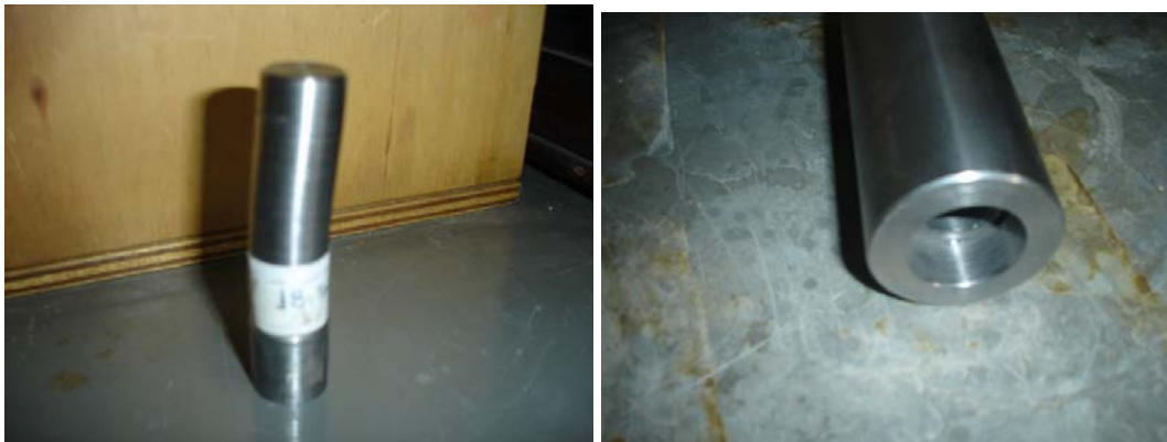
Figure 2 - Sight of the first developed matrix (deformation suffered after the first produced samples)
