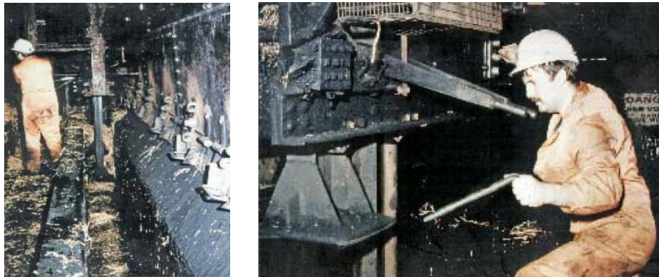
Figure 1. Stamping the coal charge at Coed Ely Coke Plant, South Wales, UK. Left: On the right are coal flaps, which are opened to allow the coal to fall into the box; straw on the left was manually forked in on top. Right: The cake is ready and the ram/charger is about to move off. The workman with the bar secures the cake in its raised position.
