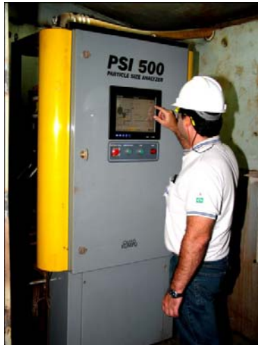
Figure 4. Laser scatter on-line particle size analyzer for monitoring hematite concentrate particle size and surface area. (2)
