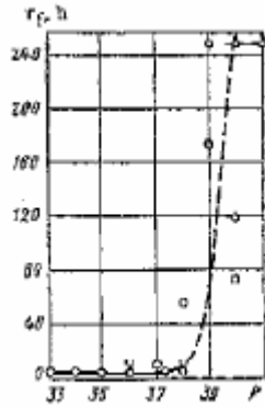
Figure 9. Correlation of hydrogen embrittlement of 18Kh1G1MF steel to the Holloman-Jaffe parameter.
