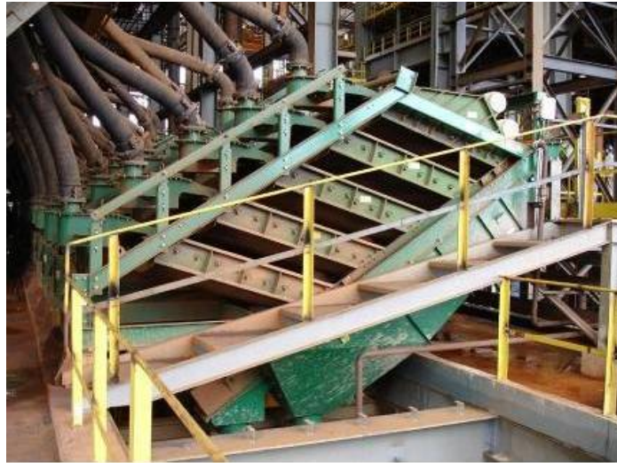
Figure 1. One of 38 Stack Sizer screening machines operating at an iron ore mine in Brazil.
