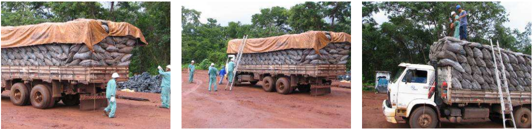
Frame volume measurement of coal in sacks – Brazil
