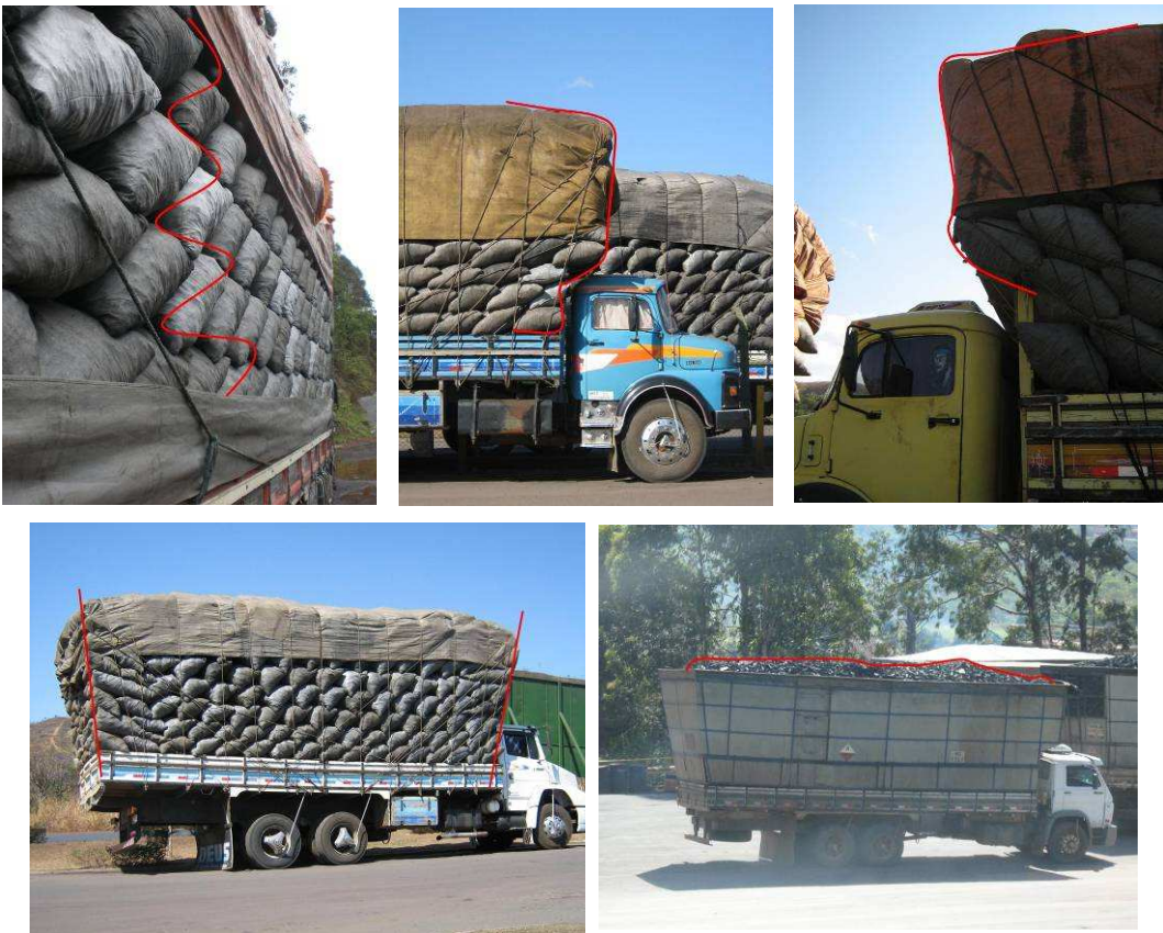
Coal load irregularities - Brazil
