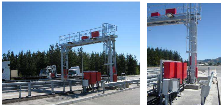
Coalmeter ® system for the volume measurement of loose coal and coal in sacks
