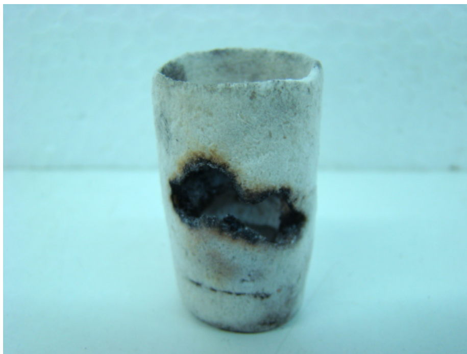
Figure 5 shows a melted crucible
