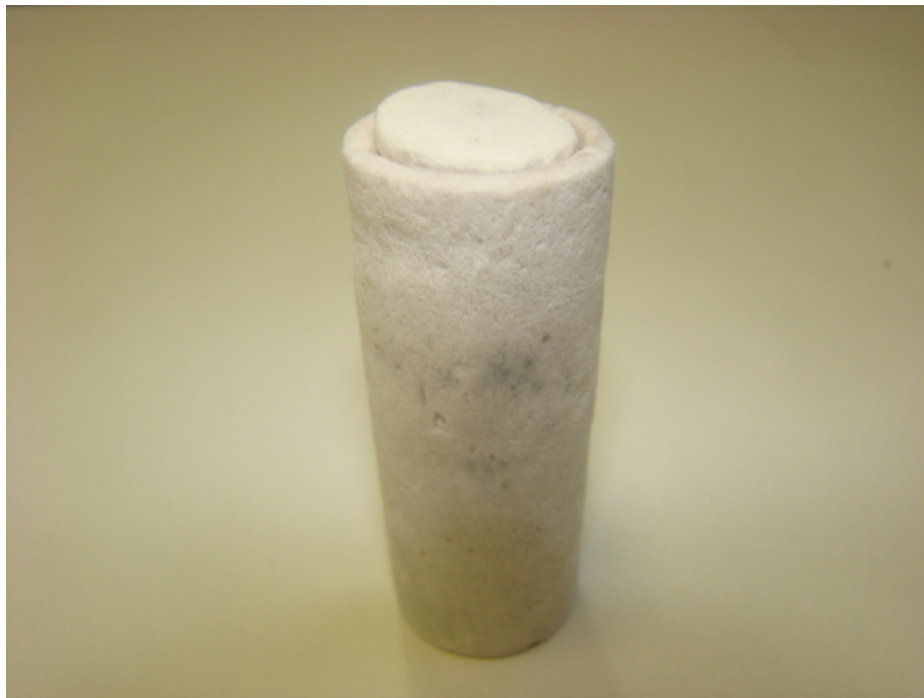
Figure 4 shows a crucible and its caps, also from ceramic fibers
