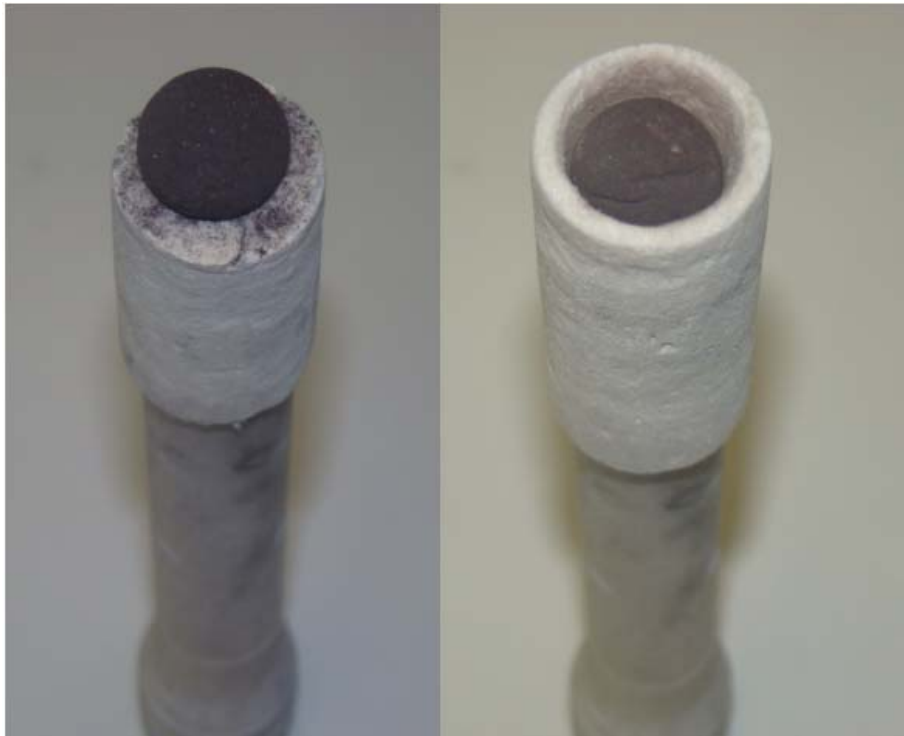
Figure 3 shows two pellets, one without a crucible and other with an open crucible
